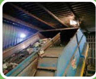
The items are tipped onto a conveyor belt and go through magnets, optical sorting equipment, and quality checks by hand to separate the material.
